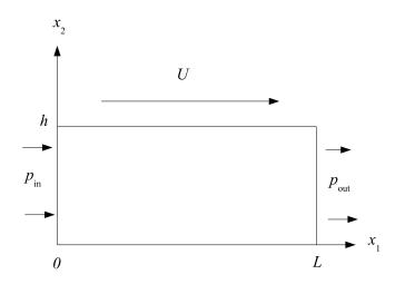
Figure 5.1: Shear flow of a viscous fluid.
