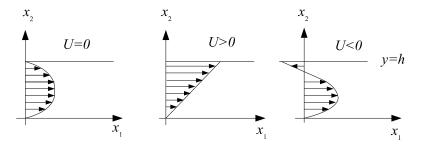
Figure 5.2: Shear flow of an inviscid fluid.
