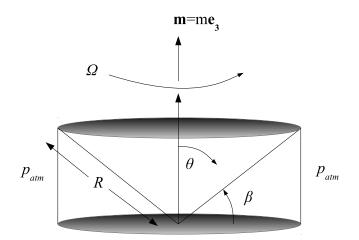
Figure 6.7: Schematic representation of the cone and plate rheometer. The angle  $\beta$  is commonly less that 10 degrees.
