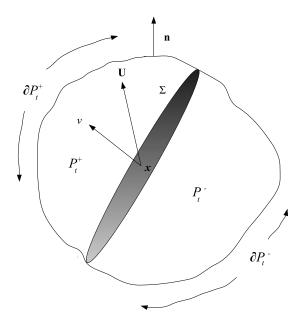
Figure 2.4: Jump conditions and singular surfaces.
