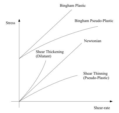
Figure 6.1: Shear-strain relation of some non-Newtonian fluids.
