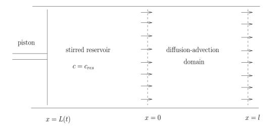
Figure 1.2: Injection of a solution from a well stirred reservoir.
