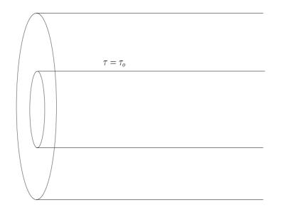
Figure 5.4: Bingham flow in a cylinder exhibiting the undeformed core.
