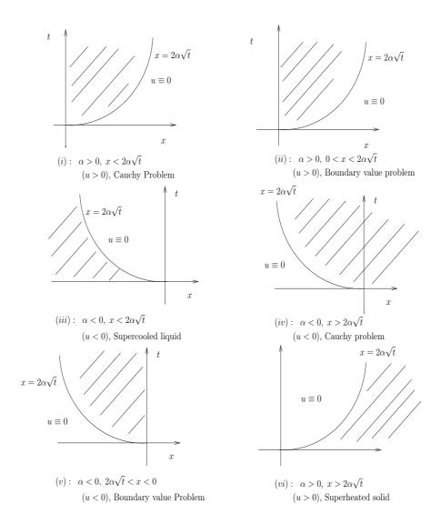
Figure 3.1: Self-similar solutions for melting (i), (ii); solidification of a supercooled liquid (iii); solidification (iv), (v); melting of a superheated solid (vi).
