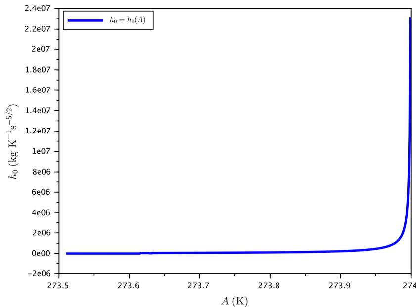
Fig. 8. Coefficient  $h_0$  characterizing heat transfer under convective conditions as a function of  $A$ .
