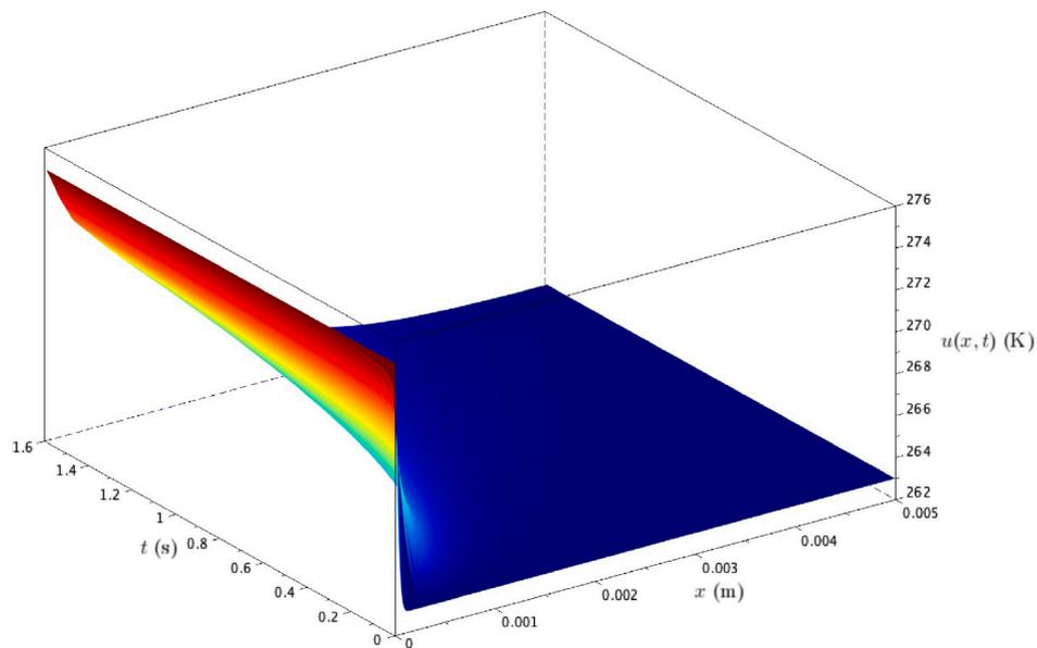
Fig. 4. Temperature distribution of the three-phase Stefan problem with a Dirichlet type condition.
